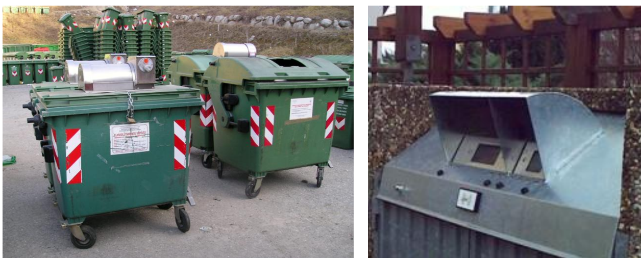
Fig. 4: MSW collection containers with lockable lids.
