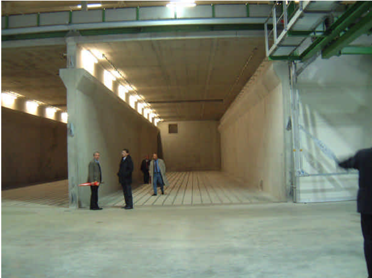
Figure 7 Example of a rotting box for the principal rotting of heavy fraction from MSW
